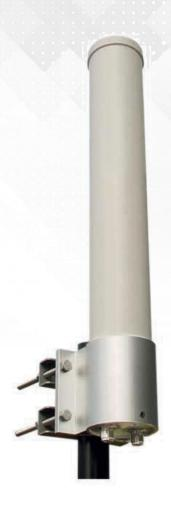
The OA05-0013 is a dual-polarity 2x2 MIMO omnidirectional antenna that operates from 5150MHz to 5850MHz. It provides a gain of 13dBi and has a VSWR of less than 2:1.It has a horizontal beamwidth of  $360^\circ$  and a vertical beamwidth of  $7^\circ$ . It is available in a UV and DC ground lightning-resistant PVC enclosure that measures  $84 \times 600$  mm and has two N-female connectors. This sector is designed for fixed and mobile deployments.
