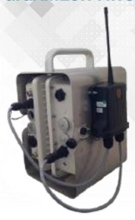
GigaMesh-AWS is a portable, autonomous, and remotely controlled WiMesh router designed to provide reliable and secure connectivity for temporary network deployment.
